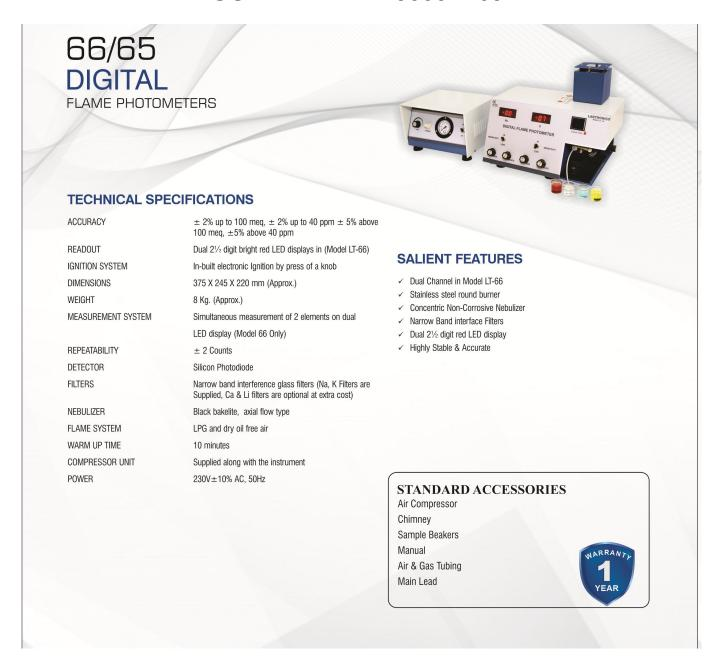
With filter (Na & K) 3 1/2 digit LED Display (ppm) along with compressor and other accessories .Ca & Li filter can be provider on request.
